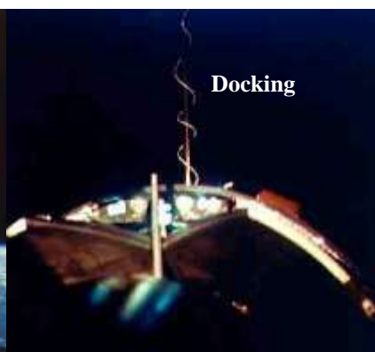
Gemini 8 and Agena-Delta T-8. After the docking, Gemini started to rotate. Armstrong stopped the rotation by disconnecting Agena and the thruster quads. Project failed.
