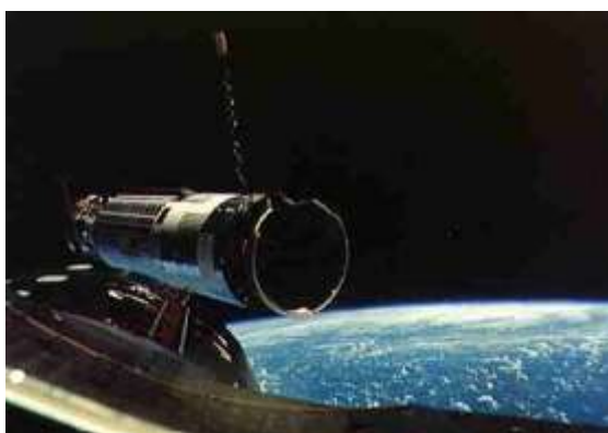
Gemini 8 and Agena-Delta T-8. After the docking, Gemini started to rotate. Armstrong stopped the rotation by disconnecting Agena and the thruster quads. Project failed.
