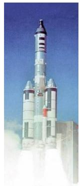
The first test flight was carried out before the programme was shut down. The Gemini ship in question was a modified Gemini 2. The MOL part was constructed from a fuel tank used on a Titan II rocket. MOL brought three satellites on this flight. The Gemini craft separated as planned from the rocket before it reached its orbit where it delivered its three satellites.
